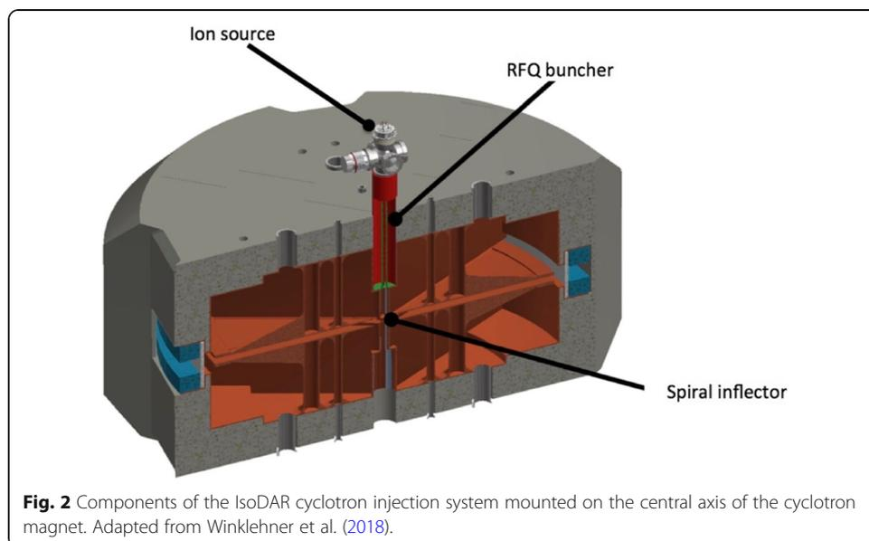
**Fig. 2** Components of the IsoDAR cyclotron injection system mounted on the central axis of the cyclotron magnet. Adapted from Winklehner et al. (2018).
