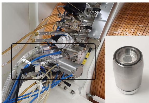
**Fig. 1** The ARTMS QUANTM Irradiation System® on the GE PETtrace (rectangular box) allowing for automated pneumatic transfer of the water-cooled target capsule (insert) containing the enriched zinc-68 on silver backing
