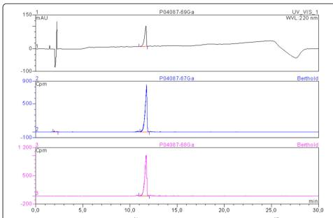
**Fig. 7** Typical HPLC chromatogram of (1)  $^{\text{Nat}}$ Ga-P04087 and radio-chromatograms of (2)  $^{67}$ Ga-P04087 and (3)  $^{68}$ Ga-P04087. (Analytic conditions: column : ACE® 100 Å C18; 150 mm × 4.6 mm, 3  $\mu$ m particle size. Gradient elution: A) H2O, 0.1% TFA; B) acetonitrile, 0.1% TFA; UV detection at 220 nm; flow: 1 mL/min; 0-2 min isocratic 5% B, 5-35% B linear gradient 20 min, 35-5% B linear gradient 2 min. Retention time (tR) for signal was 11.7  $\pm$  0.07 min
