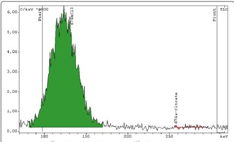
**Fig. 6** ITLC-SG of the  $^{67}$ Ga-chloride obtained by the elution of  $^{67}$ Ga from Sep-Pak SI cartridge using 0.1 M HCl. Mobile phase: 0.4 M sodium acetate pH 4. Rf ( $^{67}$ GaCl3) = 0, Rf ( $^{67}$ Ga-citrate) = 1 The same retention profile was obtained when  $^{68}$ GaCl $^{3}$  eluate was analyzed using the same ITLC-SC conditions
