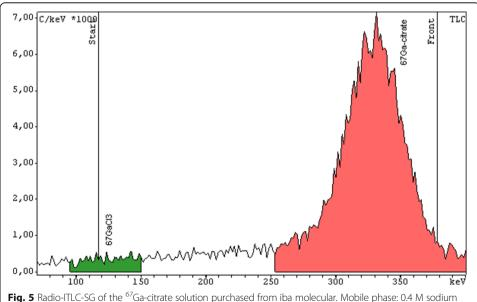
**Fig. 5** Radio-ITLC-SG of the  $^{67}$ Ga-citrate solution purchased from iba molecular. Mobile phase: 0.4 M sodium acetate pH 4. Rf ( $^{67}$ Ga-citrate) = 1
