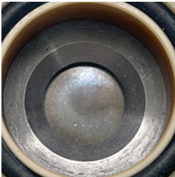
Fig. 1 Picture of foil taken ~ 1 week post irradiation (8h, 50µA, 13MeV).
