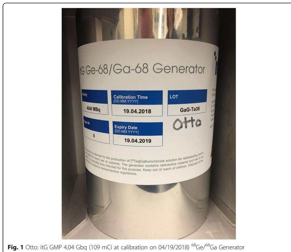
**Fig. 1** Otto: itG GMP 4.04 Gbq (109 mCi at calibration on 04/19/2018)  $^{68}\text{Ge}/^{68}\text{Ga}$  Generator
