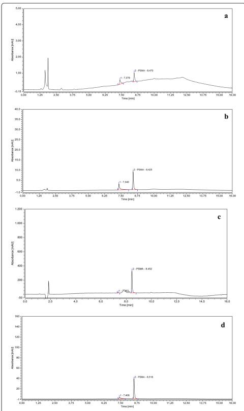
**Fig. 4** Chromatograms of 3 (**a**), 12 (**b**), and 50 (**c**)  $\mu$ g/mL PSMA-11 standard solutions injected at 3 days from preparation and chromatogram of a 50  $\mu$ g/mL PSMA-11 standard solution injected 6 months after the preparation (**d**)
