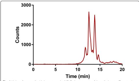
**Fig. 4** High performance liquid chromatography (HPLC) chromatogram of the radiodetector. The retention time of unbound [<sup>99m</sup>Tc]pertechnetate is 2.5 min. The retention time of [<sup>99m</sup>Tc]Tc-PSMA is between 10 and 15 min, with different peaks accounting for different protonation states
