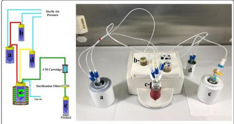
**Fig. 3** ML-Eazy fully automated synthesis device, disposable cassette and schematic flow (**a**) [<sup>177</sup>Lu] Lu vial, (**b**) Buffer and peptide vial, (**c**) Reaction vial and heater, (**d**) Saline vial, (**e**) Final product vial
