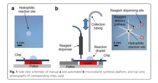
transport reagent droplets from the periphery to the center of the chip. Complete details of this setup were reported previously (Wang et al. 2017).
